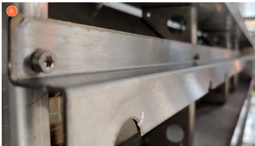
LED with bracket, mounted by means of bolts.
